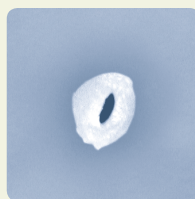
Improperly Cut Tubing
