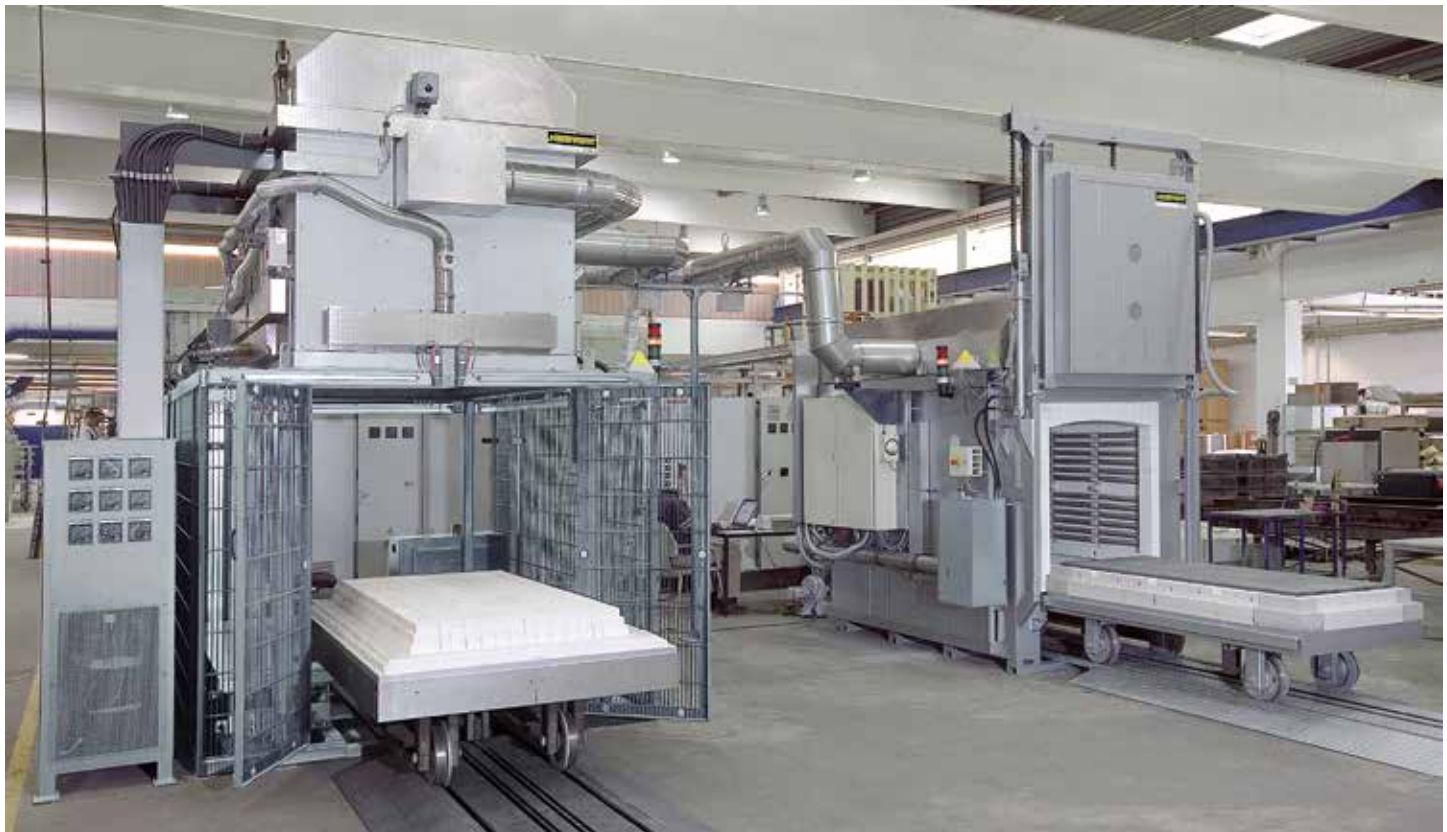
Production system consisting of a bogie hearth furnace for debinding and a high-temperature furnace for residual debinding and sintering with shared catalytic post combustion
