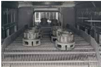
Mesh belt drive in a continuous furnace
