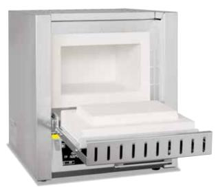
Muffle furnace L 9/11/SKM with flap door
