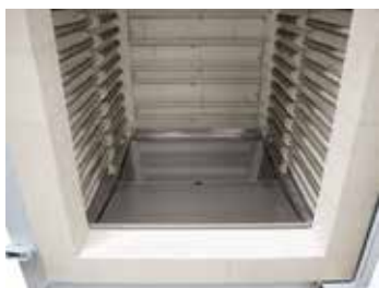
Drain pan in floor
