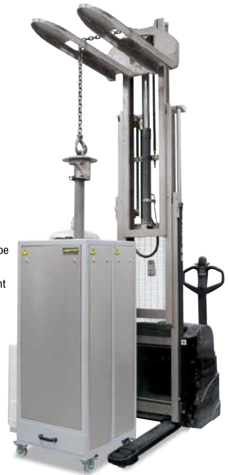
Furnace SRO 170/1000/11 with suspended pipe
