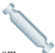
U-322 VICI® (Valco) Compatible ZDV Union 0.020" thru-hole for 1/16" OD tubing
