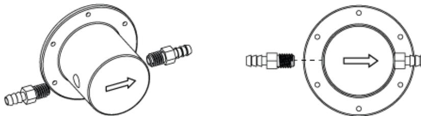
2. Screw the pump head to the fixing case of the drive.
