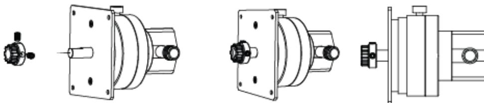
2. Mount the pump head (**NOTE:** The scale of the red flow control ring must be pointing upwards):
