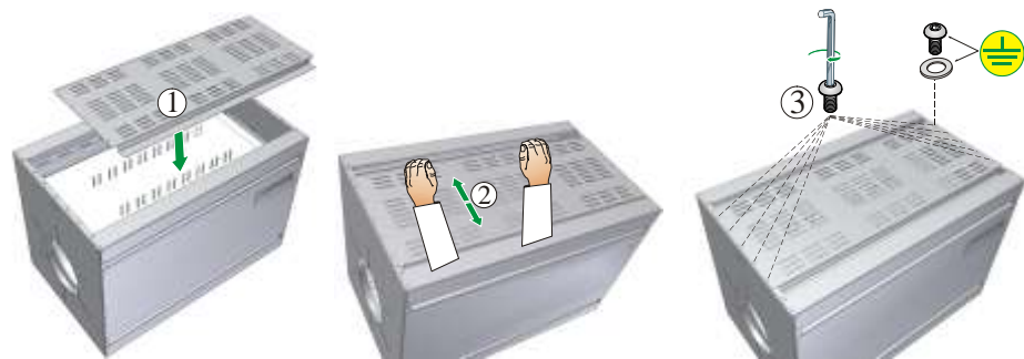
Fig. 44: Installing the Furnace Lid
