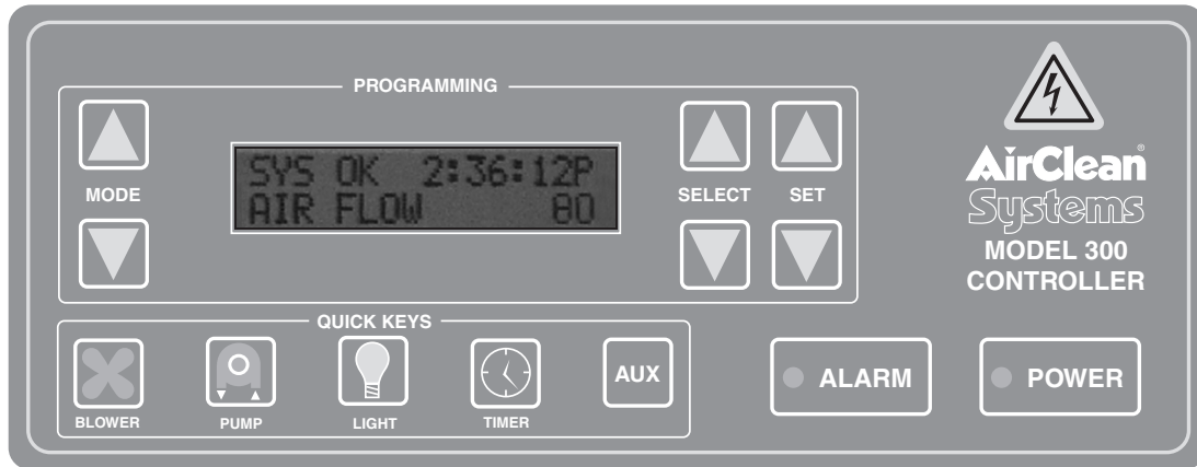
Figure 6, AirSafe™ automatic safety controller layout.
