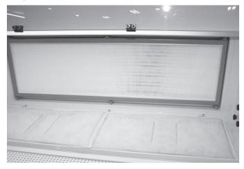
Figure 11. AC740C Pre-filter and HEPA filter.
