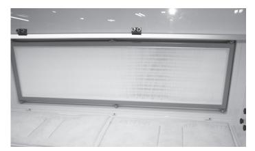
Figure 9. AC740C Pre-filter and HEPA filter.
