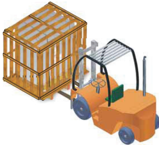
Fig. 7: Forklift prongs are pushed completely beneath the transport frame
